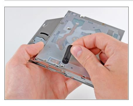
Peel off the strip of black tape covering the optical drive thermal sensor.
