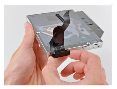
Disconnect the optical drive cable by pulling its connector away from the body of the optical drive.
