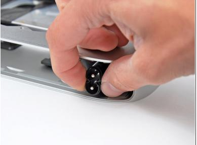
Rotate the AC-In connector 90 degrees counter-clockwise.
