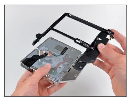
Remove the optical drive bracket from the optical drive, minding any cables that may get caught.
