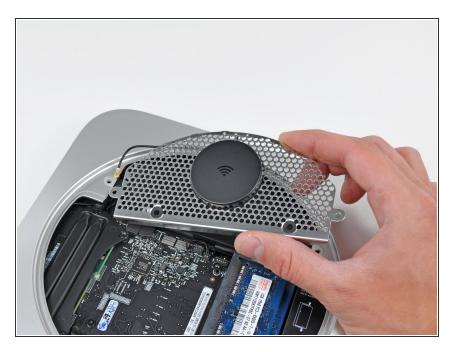
Remove the antenna plate from the mini.
