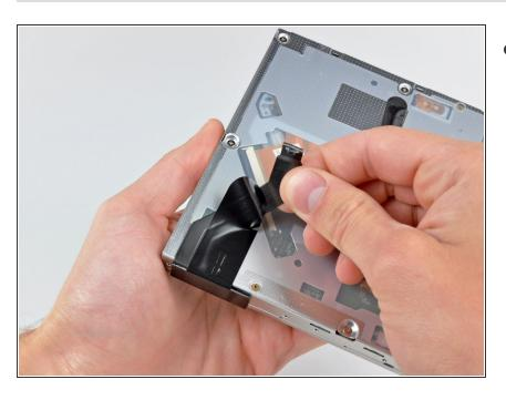
Carefully peel the optical drive ribbon cable off the body of the optical drive.
