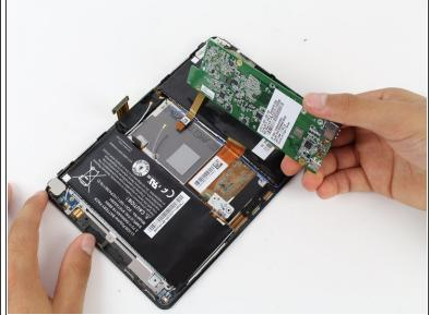
Gently lift the motherboard away from the device. If there is any resistance, check the previous steps to ensure that all connections have been removed.
