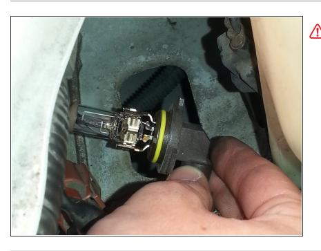
Be very careful twisting new bulb into electrical connection as the bulbs are very easily damaged.
