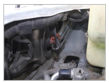
Located right behind the headlight is a red Deutsch connector. Push down on that connector to unplug wiring and rotate unconnected portion counterclockwise, facing from the driver's view, to remove bulb.
