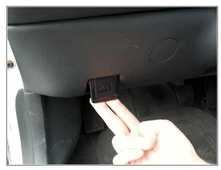
(i) Reach underneath the panel below the steering column and pull the black lever to unlock hood. The lever will have an icon of a car with a propped open hood.
