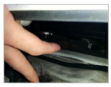
Place two fingers underneath hood but directly on top of Toyota emblem to locate hood latch. Push up with both fingers to unlock latch.
