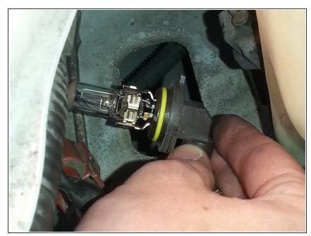
i With bulb exposed, twist broken bulb counterclockwise to unscrew from electrical connection. Screw in new bulb clockwise and replace back into socket.
