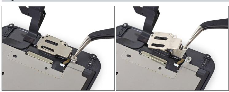
• Remove the earpiece speaker/front-facing camera bracket from the front panel.
