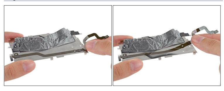
• Carefully peel the home button cable up off of the adhesive holding it to the LCD shield plate.
