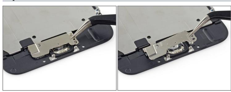
• Remove the home button bracket from the front panel.
