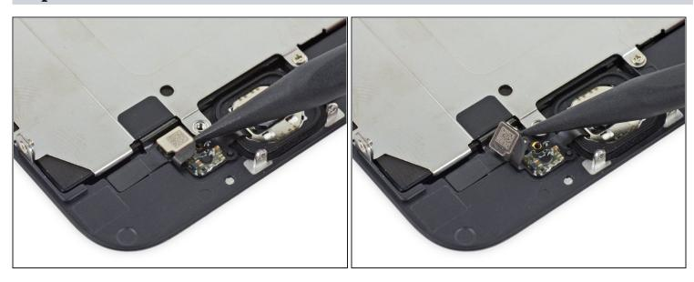
• Use the point of a spudger to disconnect the home button cable connector by pushing it up and away from the home button.
