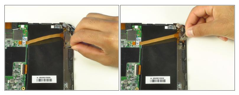
• Remove the sticker holding the touchscreen controller in place to free it from the mid-frame.
