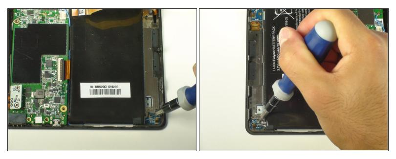
• Unscrew the small blue boards in each corner with the same Phillips screwdriver.
