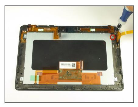
• Remove the one remaining Phillips screw holding the display in place.
