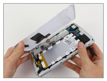
Once the backing has been pried off all around the device, remove the white backing.
