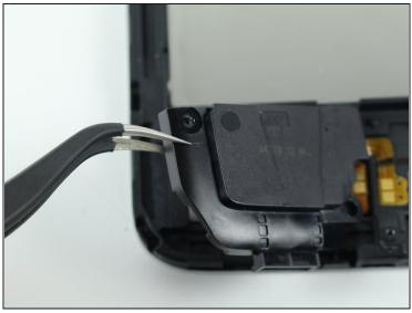
After detaching the connector and removing the screw, carefully remove the right speaker using <u>tweezers</u>.
