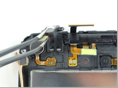
Once the connector is removed, carefully remove the headphone jack using the tweezers.
