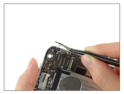
Carefully grasp the antenna clip with a pair of tweezers and remove it from the iPhone.
