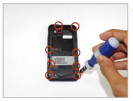
Remove eight 4mm and one 5mm Torx screws.
