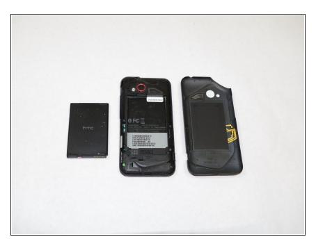
• Remove the battery after taking off the cover.
