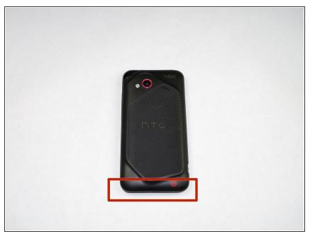
Use the plastic opening tool to pry off back cover by inserting opening tool in the space indicated and pushing down on the handle of the tool.
