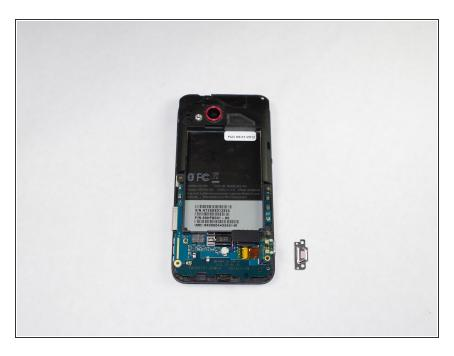
Remove the silver bracket holding the charging port in place.
