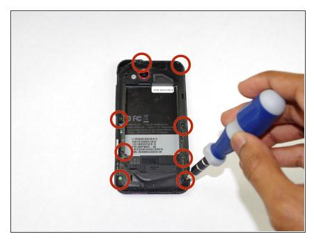
Remove eight 4mm and one 5mm Torx screws.
