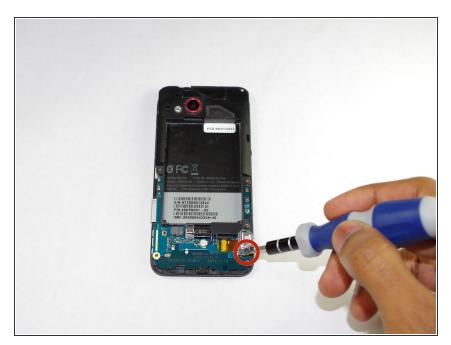
Remove the 4mm Torx screw holding the charging port to the phone.
