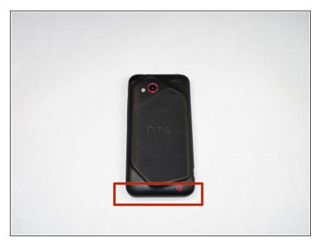
Use the plastic opening tool to pry off back cover by inserting opening tool in the space indicated and pushing down on the handle of the tool.
