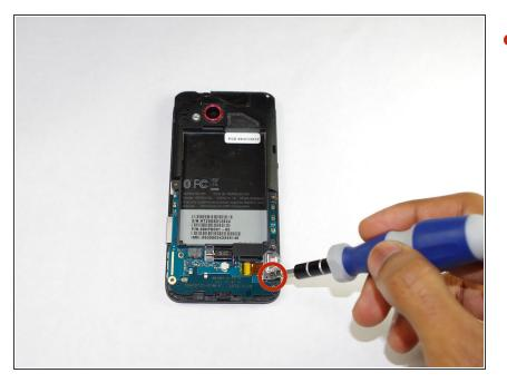
Remove the 4mm Torx screw holding the charging port to the phone.
