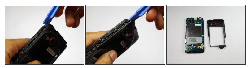
• Pry off and remove the back cover
