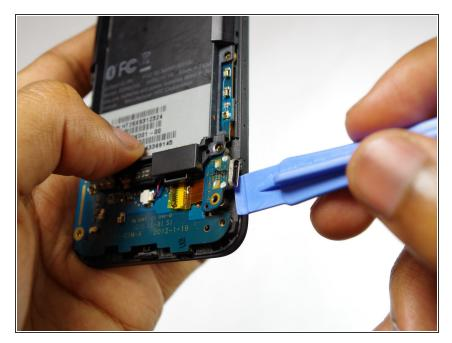
• Use a prying tool to remove the charging port as shown.
