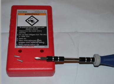
• Unscrew the two 9mm screws on the back panel using a #0 Phillips screwdriver.
