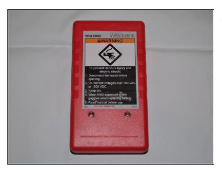
Place the meter face down, and the back panel and screws can be seen.
