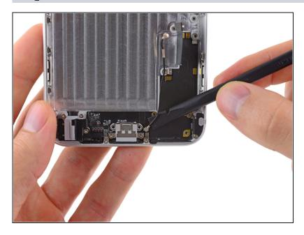
Use the flat edge of a spudger to pry the antenna connector cable up off its socket on the Lightning connector assembly.
