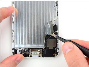
• Grasp the antenna connector with a pair of tweezers and carefully begin de-routing it from its channel on the speaker.
