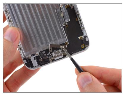
Use a pair of tweezers to lift and remove the metal bracket out of the iPhone.
