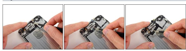
• Continue gently peeling the power button cable off the rear case and remove it from the iPhone.
