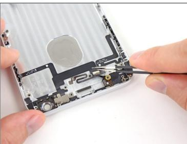
• Use a pair of tweezers to peel the single adhesive tab that resides on top of both the power button and audio control/rocker switch cable connectors.
