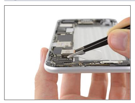
Carefully lift and remove the rear-facing camera out of the iPhone.
