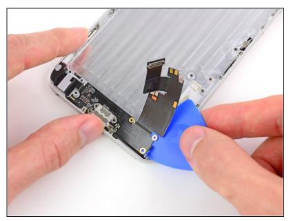
Insert the pick underneath the right bottom corner of the Lightning connector and headphone jack cable.
