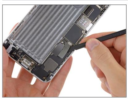
Pry the vibrator connector cable up from its socket on the logic board with the flat end of a spudger.
