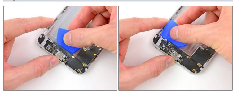
• Run the opening pick across the top of Lightning connector and headphone jack cable to loosen the adhesive securing it to the rear case.
