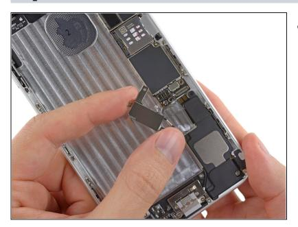
• Lift and remove the vibrator out of the iPhone.
