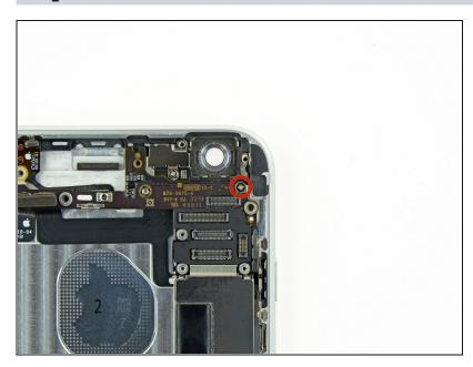
• Remove the single 1.6 mm Phillips #00 screw securing the antenna clip to the rear case.
