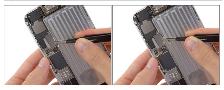
• Grasp the interconnect antenna cable with a pair of tweezers and carefully deroute it from its channel on the speaker assembly.
