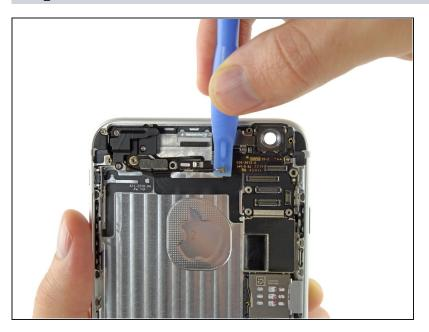
Carefully pry the antenna connector up off the logic board with a plastic opening tool.
