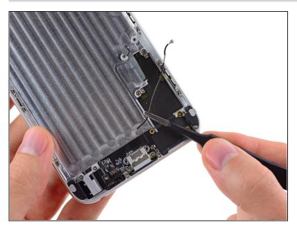
• Lift and remove the antenna connector out of the iPhone.
