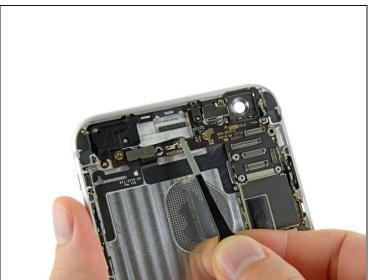
Grasp the antenna connector with a pair of tweezers and gently lift it from its retaining clip on the logic board.
