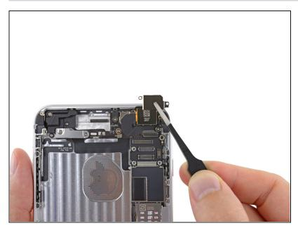
• Lift and remove the rear-facing camera bracket out of the iPhone.
