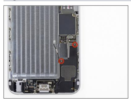
• Remove the two 2.5 mm Phillips #00 screws securing the vibrator to the rear case.
