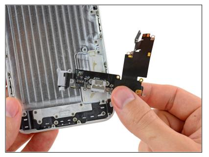
Lift and remove the Lightning connector and headphone jack cable assembly out of the iPhone.
