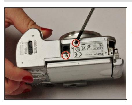
Remove the two indicated .2mm screws using a Phillips #00 screwdriver.
