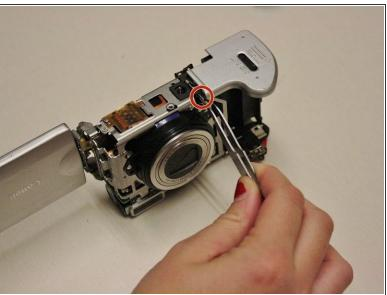
Using tweezers, gently pull remove the small rod in the battery door hinge.
