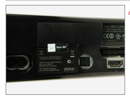
Opening your Xbox 360 any further will require breaking or removing the warranty sticker on the outer case. Your Microsoft warranty for any components not directly attached to the logic board will likely be voided by removing this seal.
