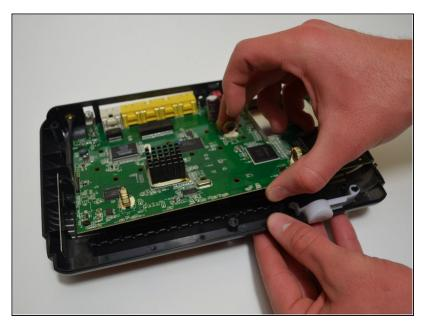
• Lift the front of the circuit board up from the bottom casing.
