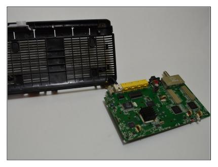
Pull the circuit board towards you until it is separate from the bottom casing.
