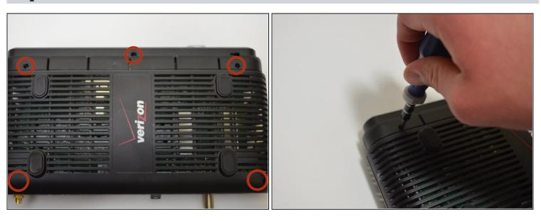
Unscrew the five 10-mm screws on the bottom of the router using a Phillips #0 screwdriver.
