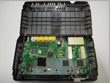
• Use a plastic-opening tool and pry the top casing from the bottom casing to expose the circuit board in the bottom half of the device.
