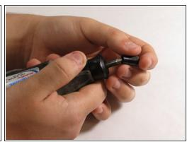
Hold down the collet lock, remove the chuck cap from the top of the Multipro by screwing counterclockwise.
