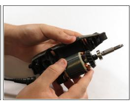
Gently lift the motor shaft out of the Multipro.
