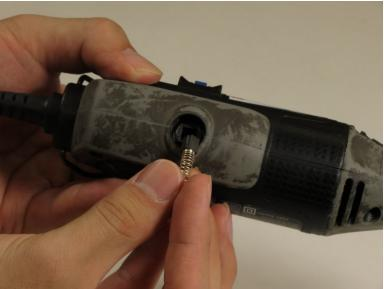
Carefully remove the carbon brushes attached at the end of the springs by gently pulling on the springs using your hands.
