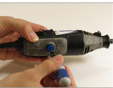
Remove the blue caps located on either side of the MultiPro, using a 3 mm flathead screwdriver.
