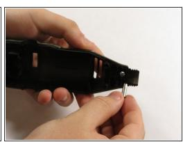
• Pull the lock pin and its casing out of the other side of the Multipro case.
