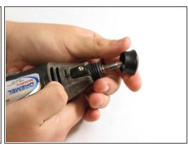
Remove the black housing cap from the Multipro located directly below the chuck cap.
