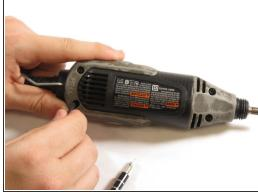
Remove the 4 screws located on the bottom of the Multipro with a T15 screwdriver.
