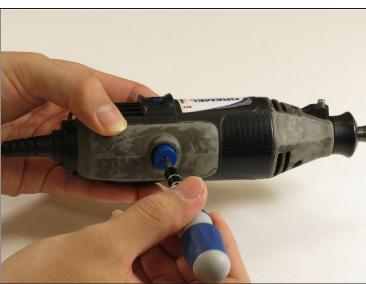
• Remove the blue caps located on either side of the MultiPro, using a <u>3 mm flathead</u> screwdriver.
