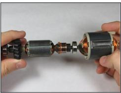
• Carefully slide the armature out of the 120V field.
