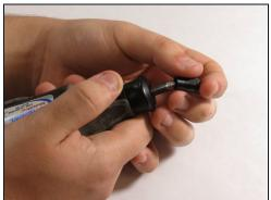
Hold down the collet lock, remove the chuck cap from the top of the Multipro by screwing counterclockwise.
