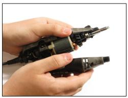
• Pull the bottom side of the casing up to remove it.
