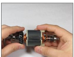
• Carefully slide the new armature back into the 120V field.
