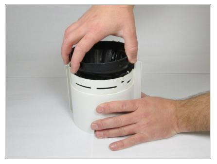
• Once the filter basket has been pried loose, grab the filter basket and lift it out of the housing.
