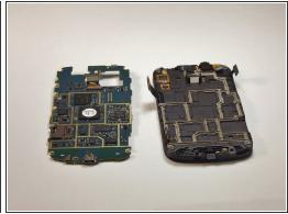
Lift the second flap to detach the motherboard completely.
