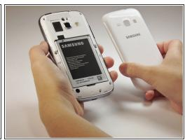
Using your finger nails or the spudger; pry the plastic casing open, and pull away from the body of the phone.
