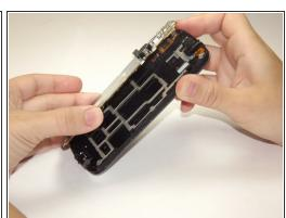
• Lift the flap up using the plastic prying tool.
