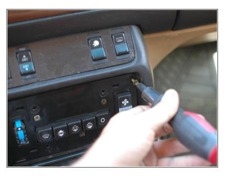
Next, remove the two screws in the upper corners of the panel behind the wood trim.
