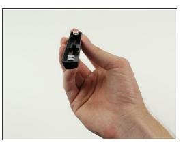
• Install the plastic rings on the new keycap. The overhang needs to be 'facing forward' so that when the keycap is placed back on the board, the overhang is furthest away from you. When attaching the new key to the board, the ends of the metal bar on the board will go through these rings.
