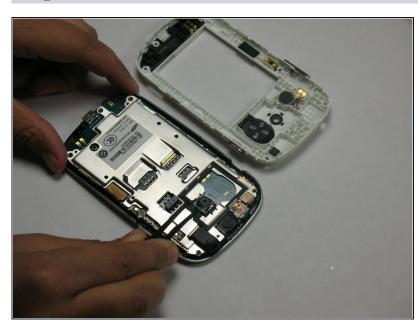
▲ Pull the camera off the system by using the <u>tweezers</u>. Perform this step with caution.
