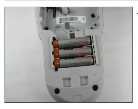
Repeat step 5 to insert the last 2 batteries.
