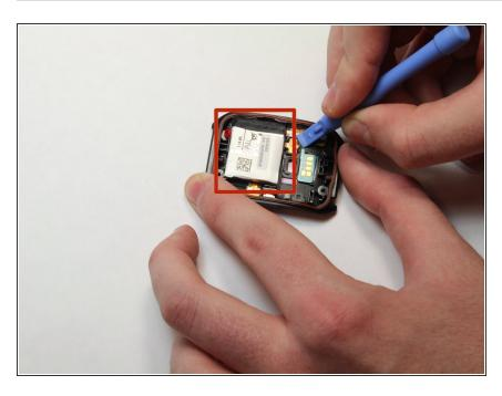
Locate the battery on the back half of the disassembled watch body. It is rectangular in shape and located just above the window for the heart monitor.
