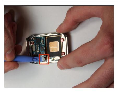
Using the plastic prying tool, gently pry away the motor's contacts and ribbon cable from the watch assembly
