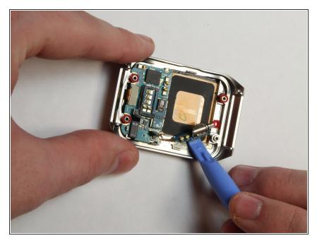
Using the plastic opening tool, gently pry up the motor.
