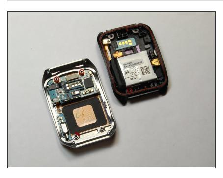
Lay both halves of the watch body assembly face down (with internal components facing up).
