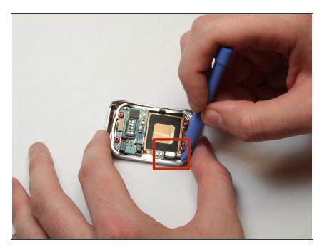
Locate the vibrator motor on the front half of the disassembled watch.
