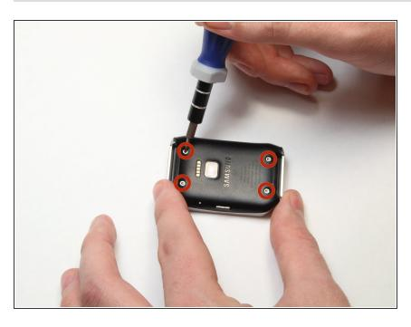
With the watch laying face-down, locate the four screws. They are located on the back of the watch, at the four corners.
