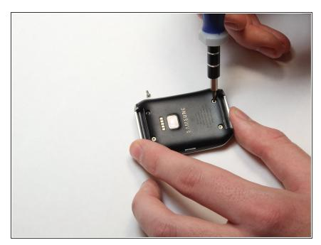
Using a Torx-T5 screwdriver, remove each of the four 4mm screws and set them aside.
