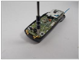
• Use the Phillips #1 screwdriver to unscrew the screws located at the bottom left and right hand corners and top of the phone; as shown in the image.
