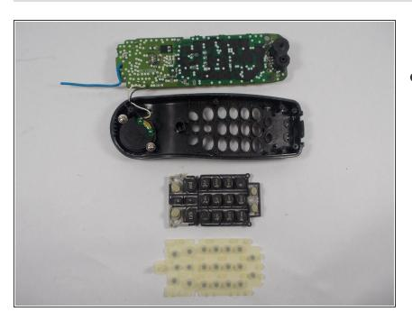
After the rubber pad is removed remove the dial pad (buttons) from the phone.
