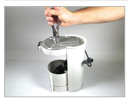
Locate the nut at the center of the base and unscrew it with a pair of basic pliers.
