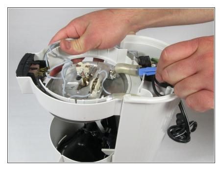
Using the larger plastic opening tool, gently push the tubing off of the oneway valve. (If the tubing is being stubborn and won't come off, run the metal spudger around the inside of tubing to free it up.)
