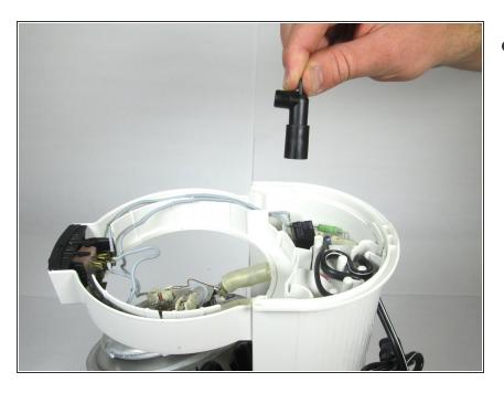
Completely remove one-way valve from the inside of the coffee maker.
