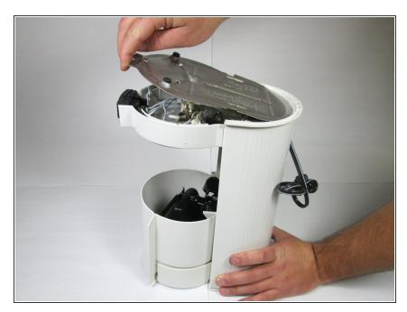
Gently lift the cover away from the bottom of the coffee maker and remove it.
