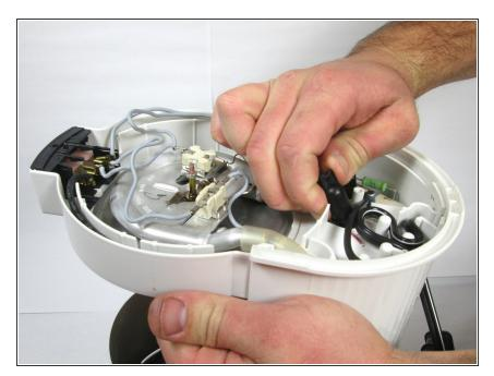
Lift up on the one way valve to snap it out of place. (This shouldn't require much force).
