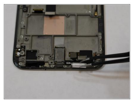
After the plastic plate is removed, tweezers can be used to remove and replace the power and volume buttons from the device.
