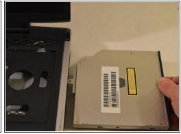
Using spudger, push the optical drive out to the right.
