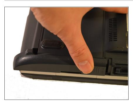
With one finger on the raised grip, slide the latch towards the front of the laptop.
