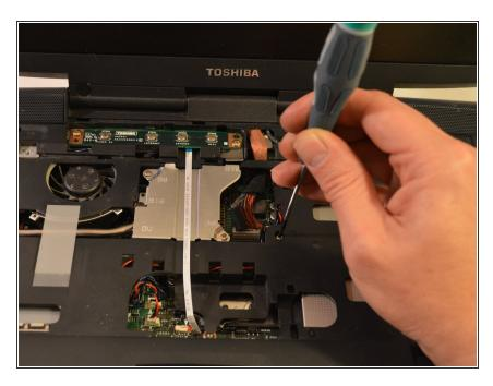
Unscrew the screw located on the left side of the optical drive near the heat sink cover in the middle of the laptop.
