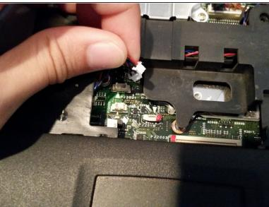
Disconnect both speaker connectors located near the center of the laptop.
