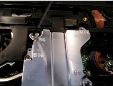
Unscrew all visible screws on the heat sink shield.
