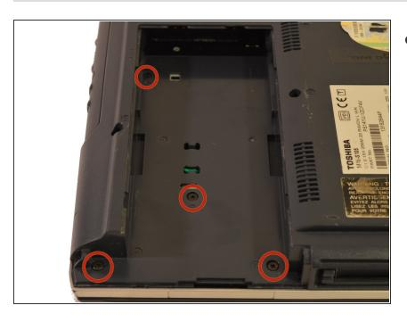
Unscrew the screws located beneath the battery.
