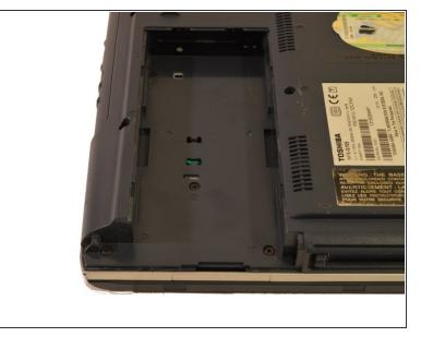
Lift the battery straight up, out of the computer.
