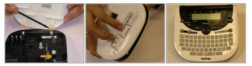
After replacing the cutter blade, you want to make sure the bottom cover is placed correctly and the two pins that lock the cover are aligned first. These pins are not a problem at the beginning while opening the cover, because they split open right away. However, you have to be careful when closing it to avoid any damage.
