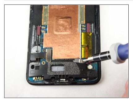
Use the Phillips #000 screwdriver to remove the single 2.7mm void screw on the bottom right.
