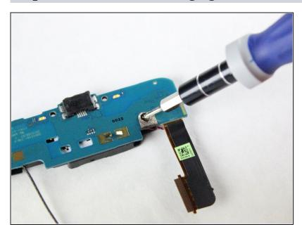
Use a Phillips #000 screw driver to remove the single 2.1mm screw located on the backside of the assembly.
