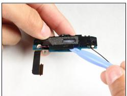
• Use the plastic prying tool to separate the assembly into two pieces: blue and black.
