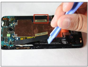
• Use your pry tool to unfasten the connectors on both sides of the motherboard.
