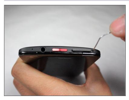
Poke a paperclip into the hole to the right of the SIM Card Tray. The SIM Card Tray will automatically pop out.
