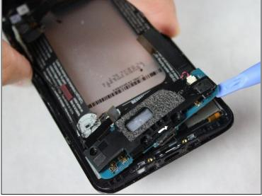
• Use the plastic prying tool to gently remove the charging port assembly.
