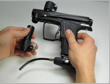
Remove the regulator by unscrewing it in a clockwise direction.
