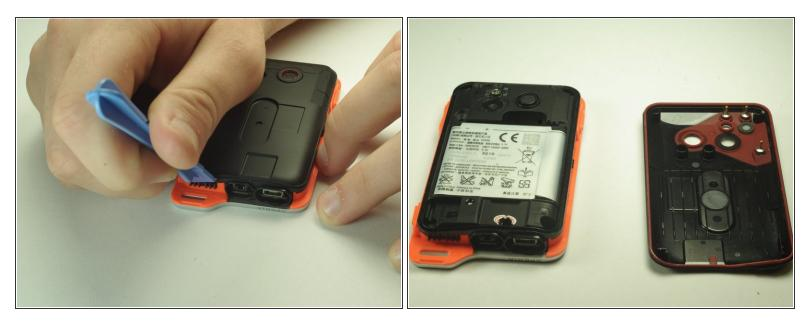
• Remove the battery shield with the plastic opening device.
