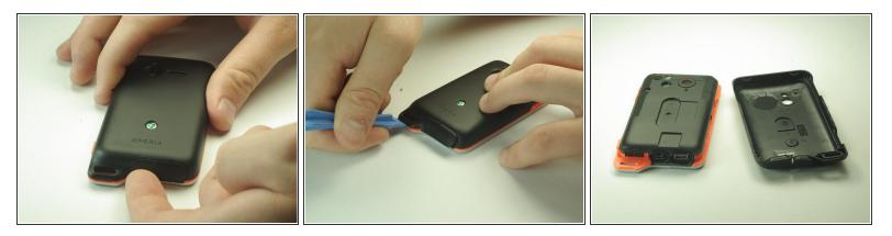
• Open the flaps and remove the back cover using the plastic opening device.
