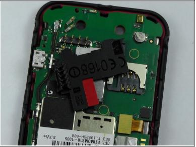
Take the metal spudger and pry the black piece, where the sim card goes, off to get to the entire antenna.
