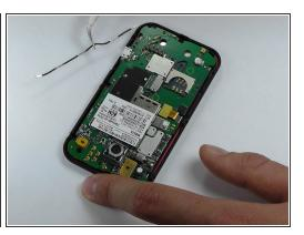
• Pry the antenna off using the metal spudger and tweezers and replace with the new one.
