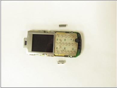
Remove the 2 clips from the sides of the phone, just below the screen with the pry tool.
