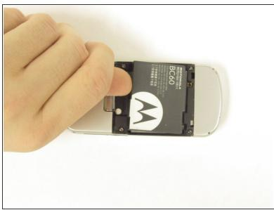
Remove the battery by pressing on the edge of the battery from the top of the phone towards the bottom and lifting up.
