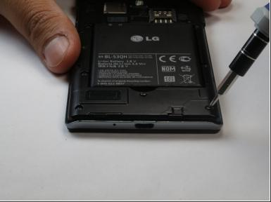
Remove the three screws from the bottom of the phone to unscrew the speaker.
