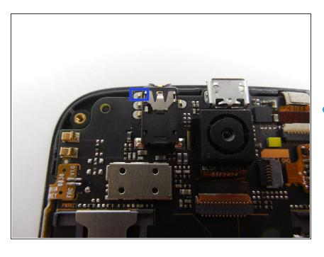
Place the solder wick over the soldered part of the first pin for the audio jack port. place the heated
