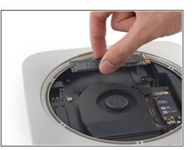
Carefully lift the SSD out of the case without scratching or touching the gold contacts.
