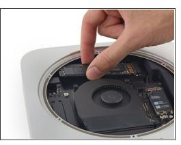
• Lift the free end of the SSD up slightly and pull it out of its socket.
