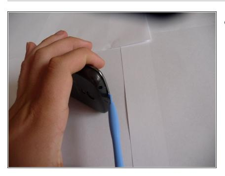
Remove the back cover with the opening tool to reveal the battery
