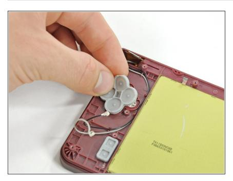
Lift the rubber pad off the back of the buttons.
