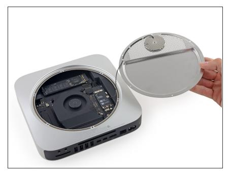
Remove the antenna plate from the Mac mini.
