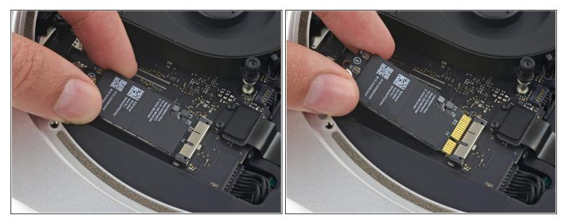
Pull the AirPort card straight out of its socket on the logic board and remove it from the Mac mini.
