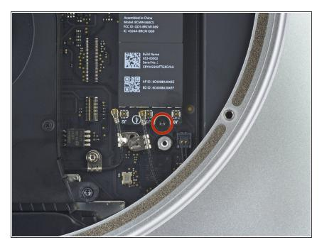
Remove the 2.7 mm T5 screw securing the AirPort card.
