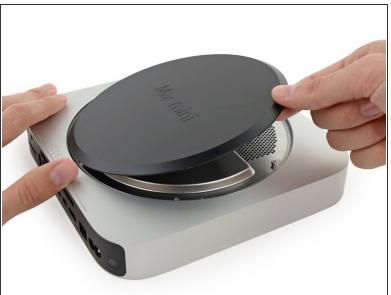
Lift and remove the bottom cover.
