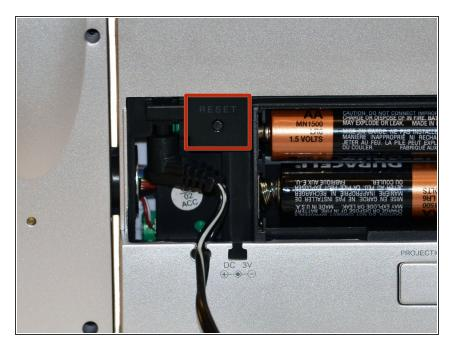
Using a pencil or other fine tipped instrument, press the RESET button. To reassemble your device, follow these instructions in reverse order.
