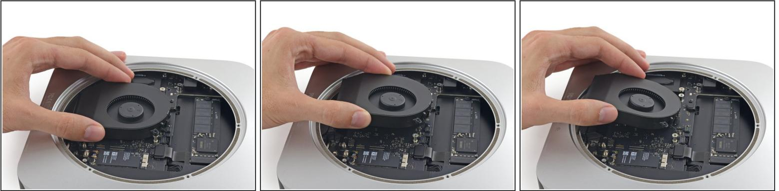
**i** The fan connector is trapped under the edge of the fan and cannot be disconnected until the fan is moved.
