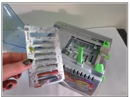
Remove the 2 screws (.75cm in length) currently securing the metal melting tray with a Phillips #2 screwdriver.
