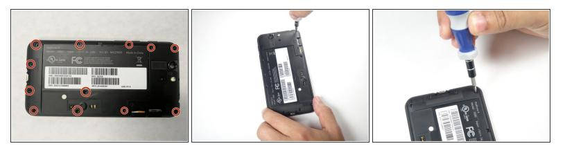
• Remove the thirteen 3.6 mm screws using the torx T5 bit in the screwdriver.
