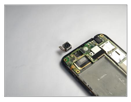
Once the camera has been pulled out, replace the old camera with a new camera.
