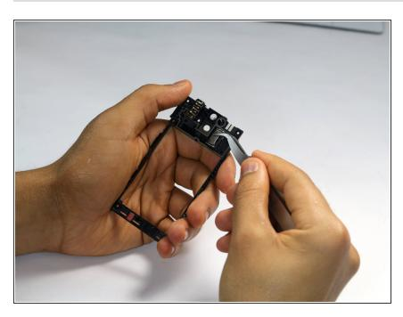
Using the tweezers, remove the loudspeaker module by firmly grasping it on one side, then slowly and carefully pulling the module in an upward direction.
