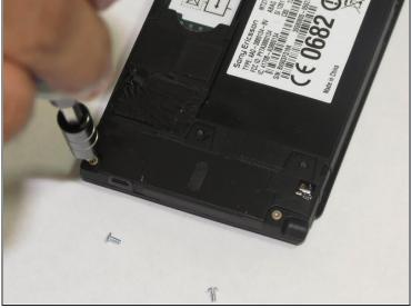
• Locate and remove the 2 additional screws, using the 26 Bit Kit, that are revealed. These are marked as shown.
