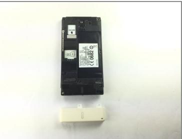
• Pry off the bottom white cover by using the opening tool as a lever.
