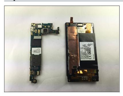
Use the spudger and slide it under the top left of the board then lift the board straight up.
