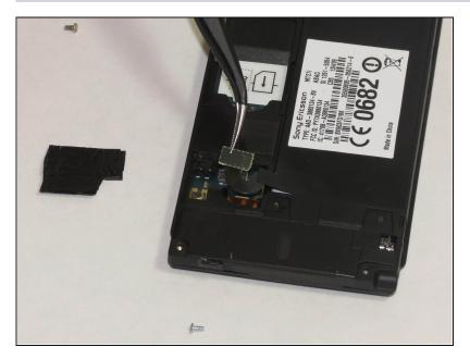
Disconnect the circuit by lifting the connector straight up as shown using the tweezers.
