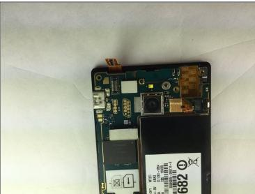
• Use the tweezers to lift up on the circuit located at the top left.
