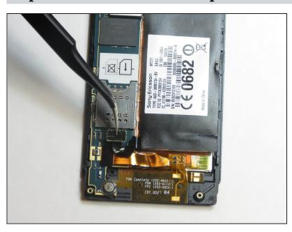
Locate the additional circuit at the bottom left. Using the tweezers, remove it gently by pulling up.
