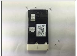
• Locate and remove the five (5) screws on the phone, using the 26 Bit Kit. The screws are at the top and the bottom of the phone as shown.
