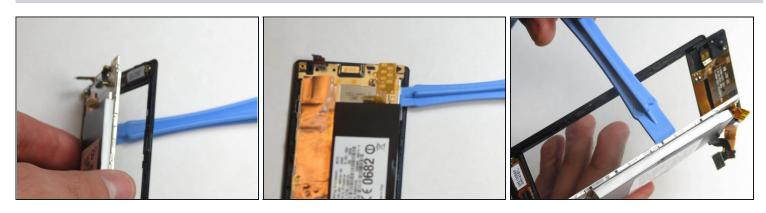
• Use either the plastic opener or the spudger to slid in the side. It will go in between the LCD screen and the spot you pulled the board off of.
