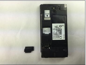
• Locate the black cover on the bottom left of phone. Use an opening tool to pry up and remove the black cover.
